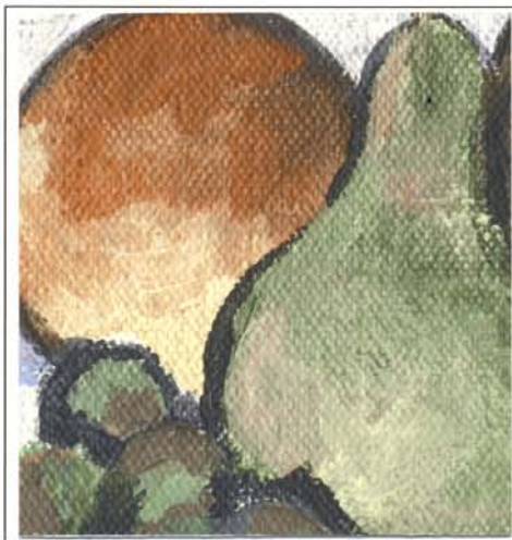
1600 Hours UV Exposure Unprotected
