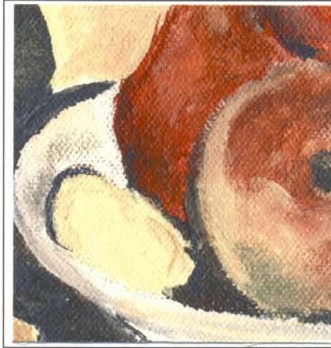
1600 Hours UV Exposure Unprotected
