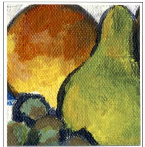
1600 Hours UV Exposure GOLDEN Gel Topcoat w/UVLS
